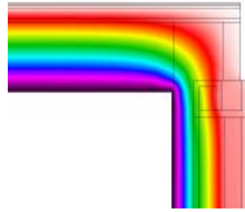
Fig. 6 Calculation of the linear thermal bridge loss coefficient. \Psi -value = 0,008 W/(mK)
